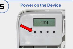
Plug in 6 ft. USB-C cable or insert 3 "D" batteries (not included) to power on.
